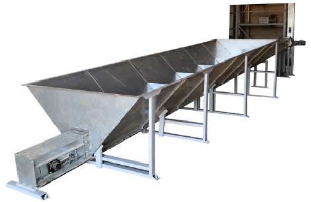
The intake pit, where all meal can be delivered regardless of chunk size
